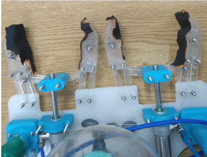
Figure 15: The Gripper's End Effectors
